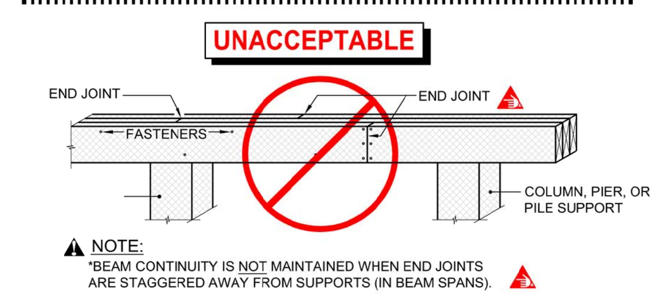
S-55 PROPER ASSEMBLY OF BEAMS NOT TO SCALE DATE: 4-9-20 Details Developed By APPIAN Consulting Engineers SEE DETAIL S-32 FOR LVL'S FASTENING SEE DETAIL S-32 FOR FASTENING SOLID SAWN MULTI-PLY BEAMS
